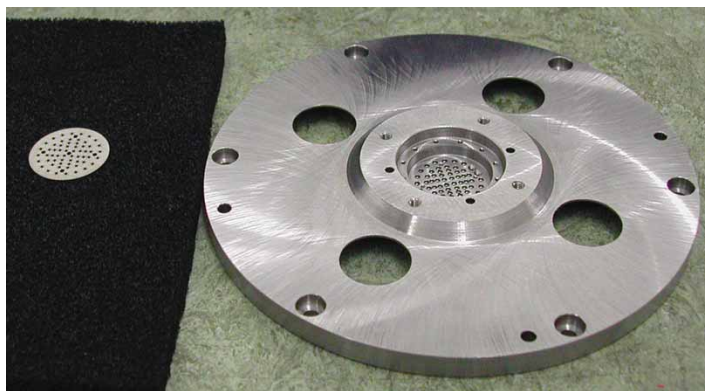
Figure 14. On the right, the rectified plate that holds the 60 ball lenses and ensures perfect alignment of the SPADA detector with the fore-optics. On the left, the clamp that keeps the ball lenses in position, just 60 \mu\text{m} above the detector. (The colour version of this figure is included in the online version of the journal.)
