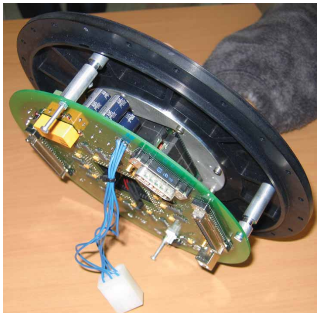
Figure 15. Complete assembled detection head, composed of the detection board, the 60 iAQCs and the SPADA detector mounted in its holder. (The colour version of this figure is included in the online version of the journal.)
