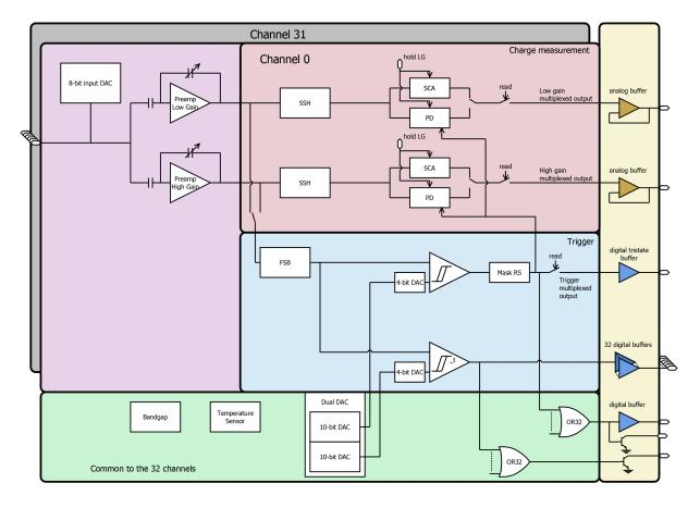
Figure 4: Architecture of the front-end CITIROC (courtesy of WEEROC).
