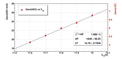
Figure 14: Gain variation in ADC units as a function of the  $V_{op}$  at 15.01°C. For clarity, the correspondent absolute value of the gain is reported on the right.
