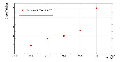
Figure 12: Optical cross talk probability versus operating voltage at  $15.01^{\circ}$ C. The error of each point is less than 0.1 %, so it is not visible in the figure
