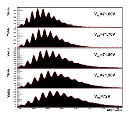
Figure 13: Pulse height distributions for operating voltages in the range (71.60-72.00)V, computed at temperature T=15.01C°C.
