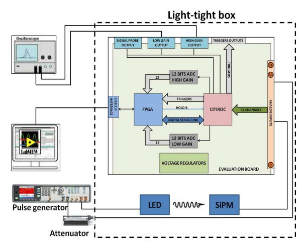
Figure 5: Schematic view of the set-up used for the SiPM+CITIROC characterization.
