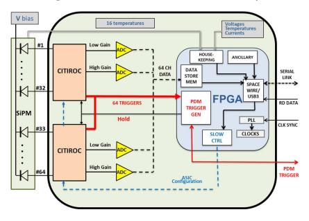
Figure 2: A schematic view of the connections to the ASICs.
