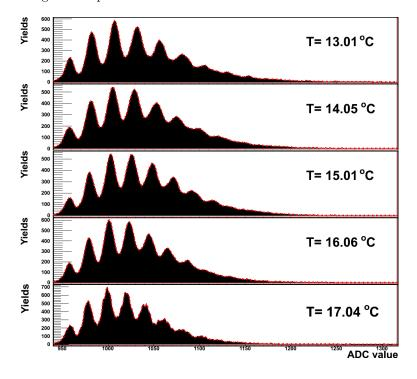
Figure 15: Pulse height distributions for several temperatures at the operating voltage of  $71.80~\mathrm{V}.$
