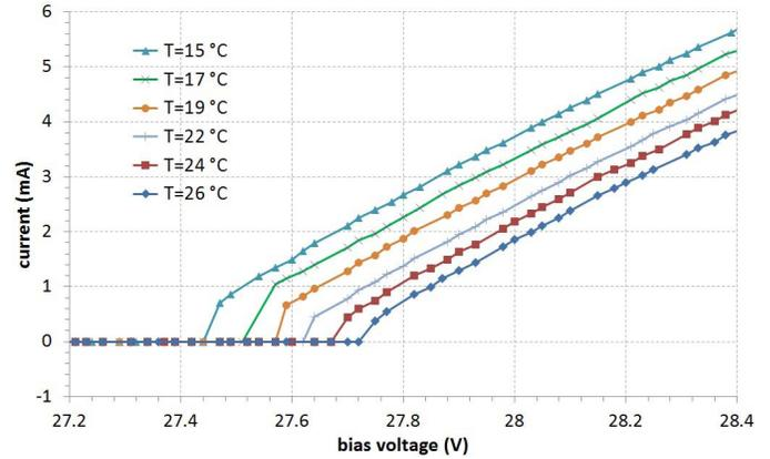
Fig. 12. Reverse current plots of a basic STM SPAD microcell as a function of the applied voltage at different operating temperatures.
