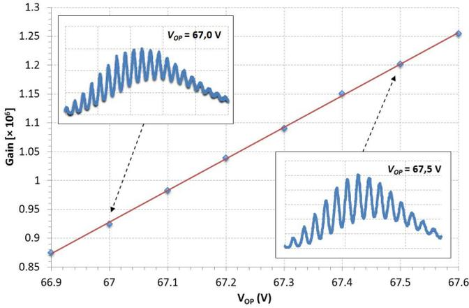
Fig. 9. Gain measurements as a function of the bias voltage for the Hamamatsu device. The linear fit allows to extrapolate the breakdown voltage.
