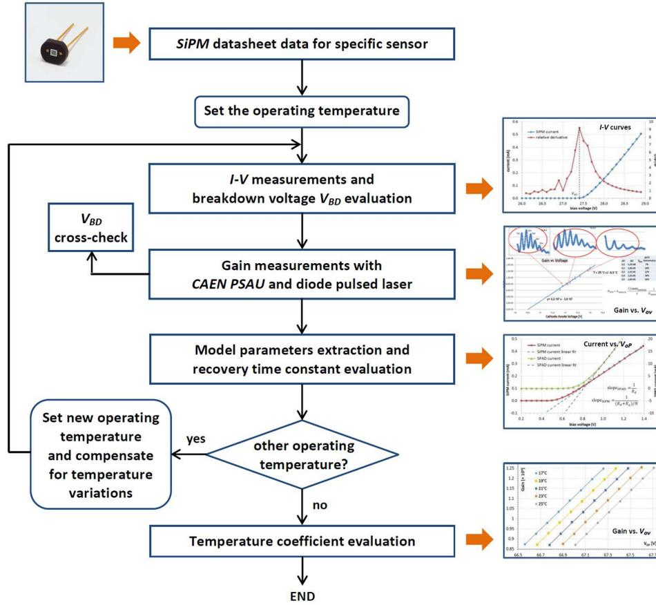
Fig. 5. Basic flow-chart representation of the adopted electrical characterization procedure for SiPM detectors.
