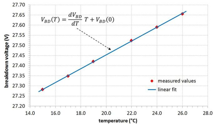
Fig. 13. Breakdown voltage variations of the single STM SPAD microcell as a function of temperature and relevant thermal coefficient evaluation.
