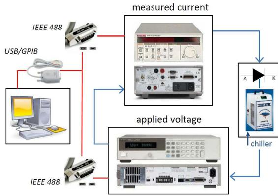
Fig. 2. Experimental apparatus used for breakdown voltage measurements with the traditional and derivative methods.
