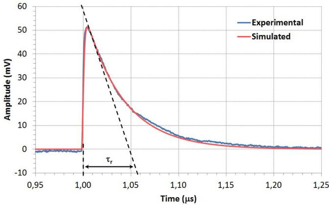
Fig. 11. Simulated and experimental output signal waveforms on a 50-Ω load resistor for the Hamamatsu MPPC device under a single firing cell.
