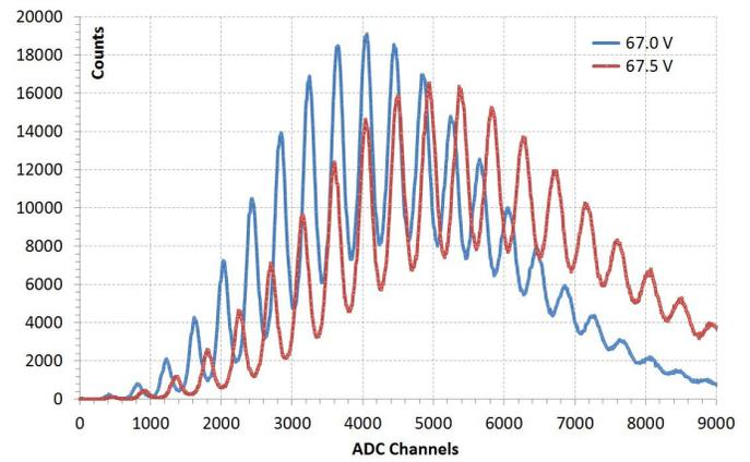
Fig. 8. Charge amplitude histograms for two different bias conditions at 23 °C for the Hamamatsu device.
