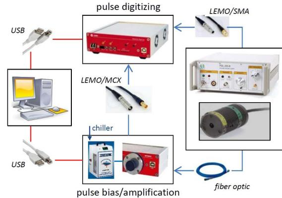
Fig. 4. Experimental apparatus used for gain measurements.
