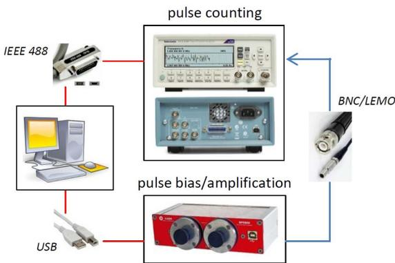
Fig. 3. Experimental apparatus used for breakdown voltage measurements with the dark count rate method.
