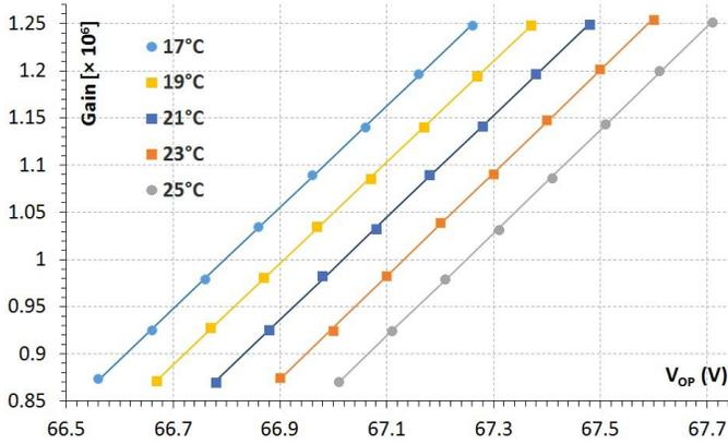
Fig. 14. Gain measurements on the Hamamatsu MPPC device as a function of the operating voltage at different temperatures.
