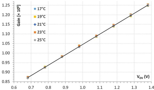
Fig. 15. Gain fluctuations for the Hamamatsu MPPC device as a function of overvoltage at different temperatures.
