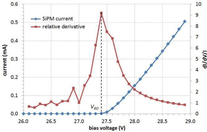
Fig. 7. Reverse STM SiPM current and relative derivative plots. The highest peak of the current derivative gives an estimation of the breakdown voltage.
