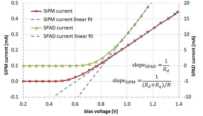
Fig. 10. Forward  $I$ - $V$  measurement plots for the STM SiPM detector and for the relevant single SPAD microcell.
