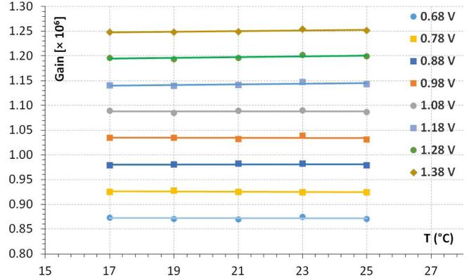
Fig. 16. Gain fluctuations for the Hamamatsu MPPC device as a function of temperature at different overvoltage.
