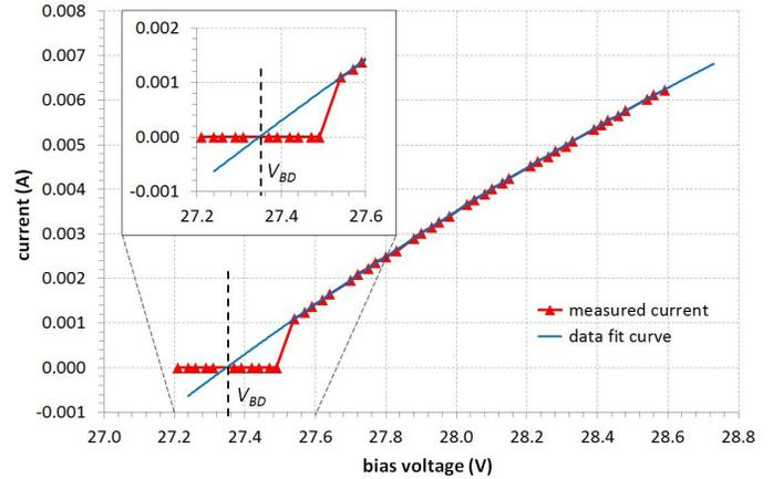
Fig. 6. Reverse  $I$ - $V$  characteristics for the single STM SPAD device at room temperature around the breakdown potential.
