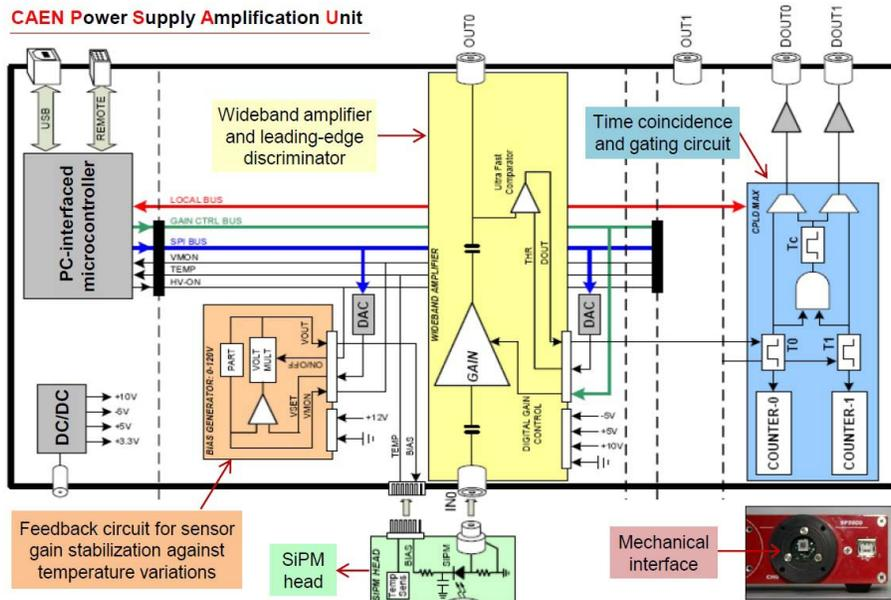
Fig. 1. Simplified electrical schematization of the CAEN power-supply/amplification unit used for the SiPM electro-optical characterization.
